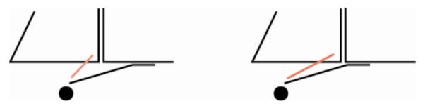
The illustration on the left is not good geometry. The tailwheel is positioned too far forward resulting in a steep angle from the rudder attachment point to the steering arm on the tail wheel. With this situation the rudder movement tries to lift the tailwheel as much as turn it. This results in poor ground handling and unnecessary strain on the rudder servo.
