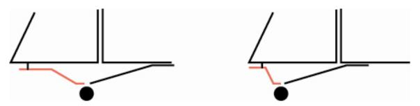
The illustration on the left is good geometry for a tiller arm steering system. The rule of thumb is the pivot point on the tail wheel should not be more than 1 ½ inches behind the rudder hinge line. If you get it further back than this you will see excessive over steer. Example; the rudder turns 30 degrees and the tailwheel turns 45 degrees.
