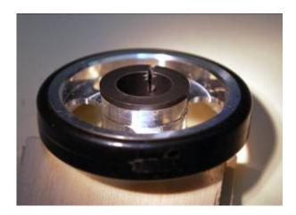
2. After you have a groove cut most of the way through take any sharp thin knife blade and slide it under the flange. At this point you should be able to pop the bushing out with a twisting motion of the knife blade. If it won't pop out cut the groove a little deeper.
